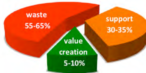
Figure 1: proportion of construction effort creating value (5-10%), supporting value creation (30-35%) and wasted (55-65%) – much of the activity that supports value creation is logistics.
